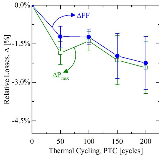
Fig. 6. Relative power and FF losses after TC with current injection of medium-area modules. Electrical properties are analyzed after 50, 100, 150 and 200 cycles.
